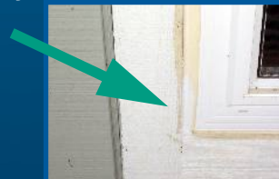
Leading brand, left exposed to sunlight for 30 days with strip of "white" to show difference
